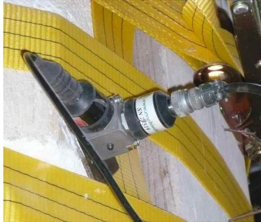
Figure 4: IEPE seismic accelerometer settled on a pillar
