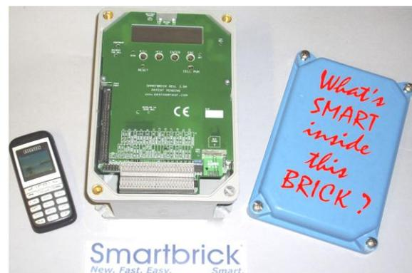
Fig. 4. "Smartbrick<sup>®</sup>" wireless autonomous SHM platform [6]
