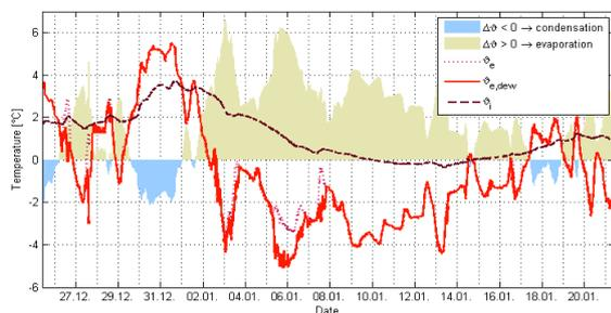
Fig. 3. Temperature measurement and dew-point calculation [5]
