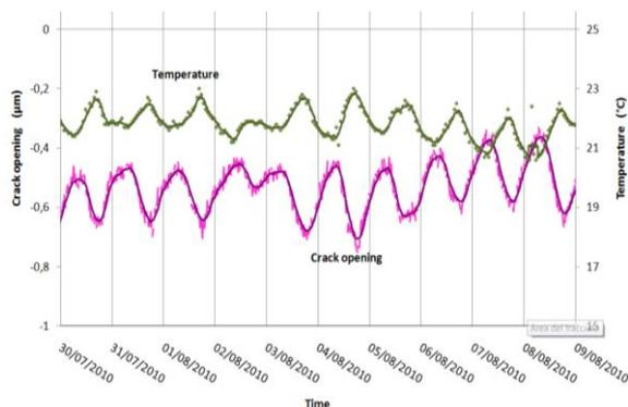
Fig. 6. Comparison of crack opening and ambient temperature [6]
