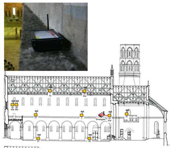
Fig. 2. Sensor node distribution and (inset) single node on a ceiling inside the Johanniskirche, Schwäbisch Gmünd, Germany [5]
